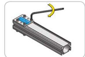
4.3. **How to tighten the screws:** The screws must be tightened but be careful not to tear the thread. The torque of the m6 screws should be between a minimum of 10 N·m (91 inch-lbs) and a maximum of 13.5 N·m (120 inch-lbs).
