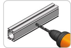
The maximum diameter of the smoothed hole must not exceed the recommended diameter. Please see the table.
