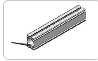
3.4. **Drilling:** during the drilling operation, it is required to have the pilot hole in the centre of the pipe. Please use a drilling jig.
