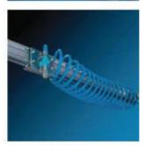
MAT is a trolley that fits directly onto the distribution line HBS 50, equipped with an outlet plate for compressed air and hanging points for balancers and tools. The pipe has the double role of rail and distributor manifold, thus reducing the overall dimensions and construction costs of an assembly line.
