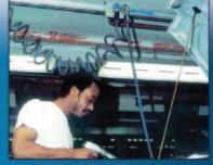
Trolleys running overhead on the aluminium pipework supporting and feeding pneumatic tools.
