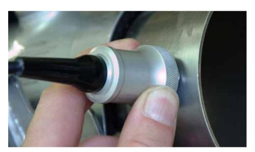
The ultrasonic thickness gauge is used to measure wall thickness, which is key information to calculate the exact inner pipe diameter.
